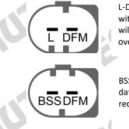
L-DFM—This alternator functions using a conventional warning light circuit with a digital field monitor signal (partially ECU controlled). The alternator will begin to charge when the warning light is extinguished but can be overridden by the DFM(ECU) controlled signal
