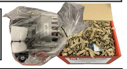
When returning a new or warranty part, if you are reusing the packaging we have provided, the alternator **must be in a sealed plastic bag** before being packed into the box. Not sealing the unit in a bag will allow the shredded cardboard in the box to contaminate the alternator meaning it will have to be stripped and reworked once we receive it.
