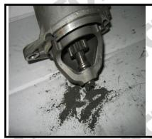
Signs of grey/metal dust can indicate that failure of the starter motor has been caused due to a failing Dual Mass Flywheel.
