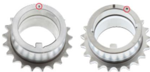
Crankshaft sprocket timing marks.
