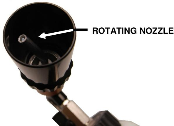
5. Press the "trigger" all the way; move the Twister slowly in circular motions over the surface you are cleaning.
