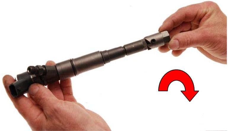
Insert the cutter into the injector
