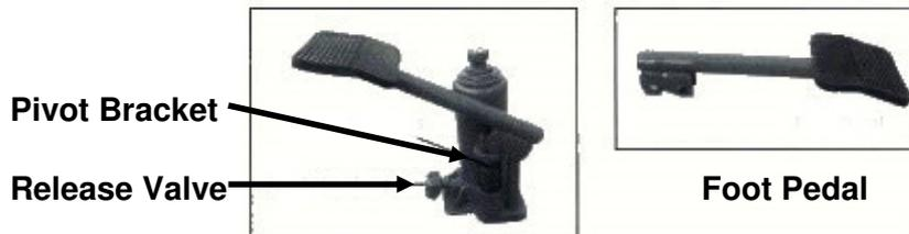
5. Raise the HDRAULIC RAM with the FOOT PEDAL insert the HDRAULIC RAM into the LIFT BASE.
