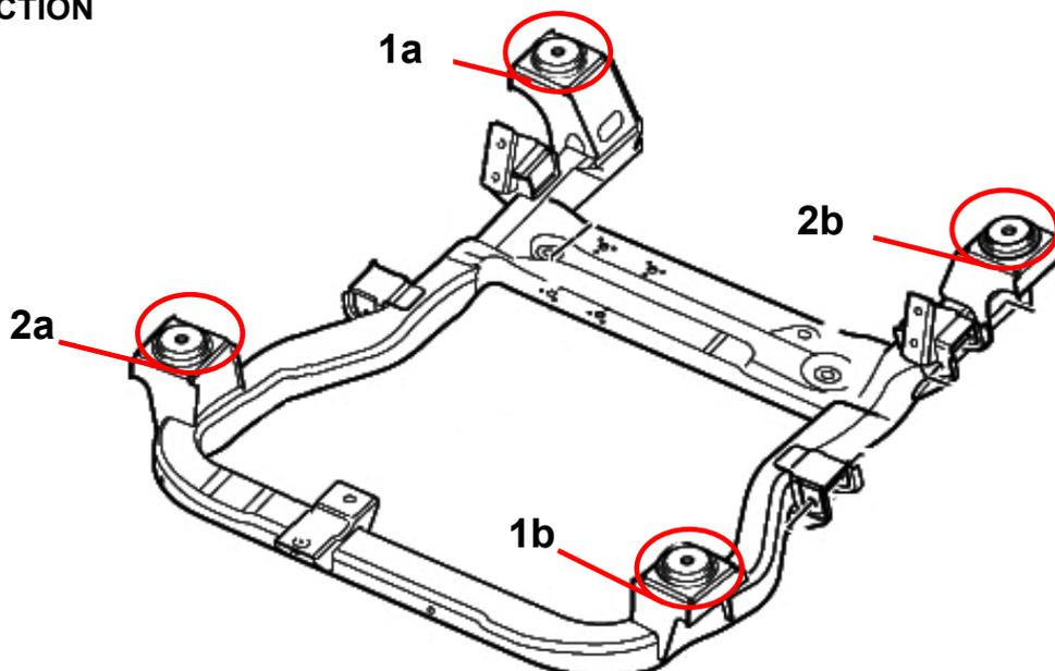
For adjustment of the subframe, the opposite screws must be successively replaced with the positioning bolts to the marked locations in 2 steps.
