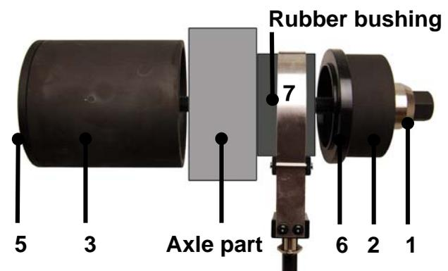
Pretension the bushing by means of the tool (7) prior to applying.
