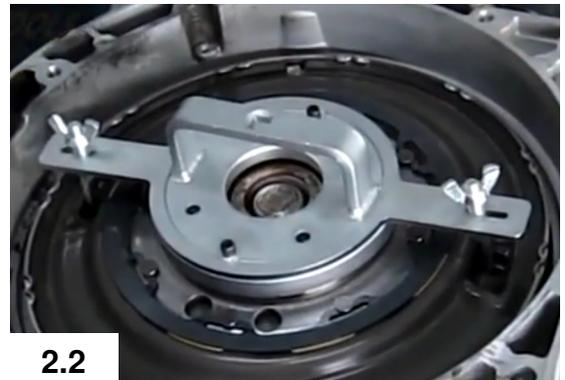
3. Loosen clutch unit by sudden turning it counterclockwise.
