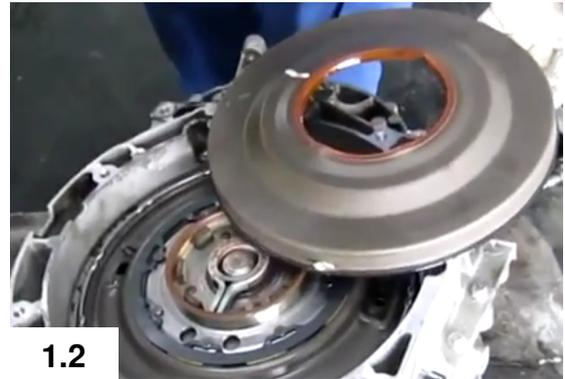
2. Remove the cover plugs (4 piece) and install the dual clutch tool.
