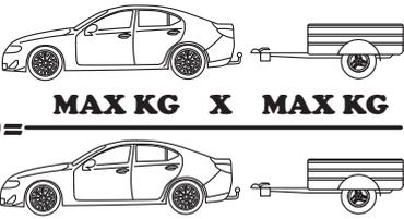
$$D = \frac{\text{MAX KG} \times \text{MAX KG}}{\text{MAX KG} + \text{MAX KG}} \times 0,00981 \leq 12,28 \text{ kN}$$
