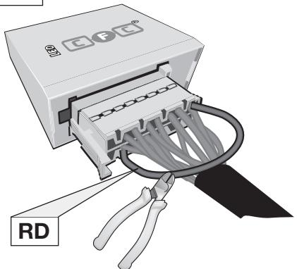
**Pin 11 and Pin 2 disconnected**
